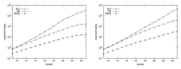
Figure 3: Average number of scanned vertices for local queries on NA with travel times (left) and distances (right). The horizontal axis refers to *buckets* with 1 000 pairs each. Each pair *s*-*t* in bucket *i* is such that *s* is chosen at random and *t* is the *j*-th farthest vertex from *s*, where *j* is selected uniformly at random from the range  $(2^{i-1}, 2^i)$ . The vertical axis is in log scale.
