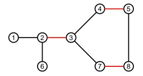
Following (1, 2, 3, 4, 5, 8, 7, 3, 2, 6), a fake augmenting path is found. False positive: an augmenting path does not exist.
