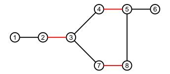
Following (1, 2, 3, 7, 8, 5), *label*(5)  $\leftarrow$  *odd* and vertex 6 is not reached. False negative: an augmenting path (1, 2, 3, 4, 5, 6) does exist.
