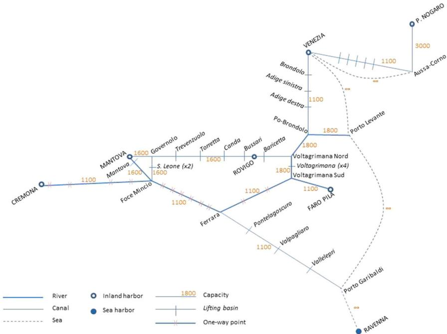
**Fig. 1** The Northern Italy waterway system network
