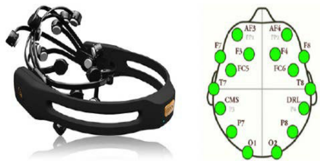
Fig. 2. The Emotiv+ system and the 14 electrodes
