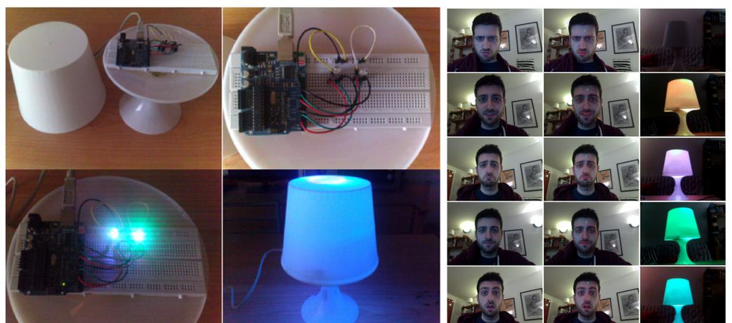
Fig.3: a) Color control: the actual color stimulus is generated through a modified Ikea lamp, where the RGB LED is controlled by an Arduino UNO board. b) Experimental results of transcoding using the Mood Lamp.
