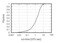
If all influential parameters are identified and fixed, the *RTD* diagram degenerates into a step function (all instances require the same time)
