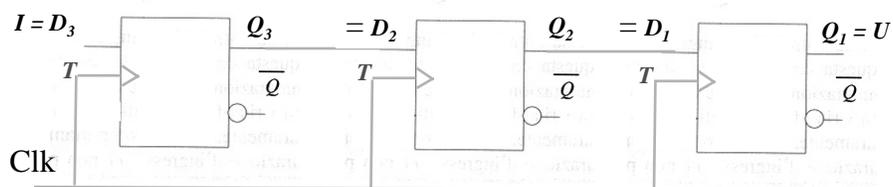
**Registro a scorrimento (shift register o barrel shifter).**
