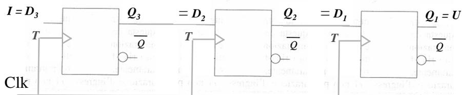
**Registro a scorrimento (shift register o barrel shifter).**
