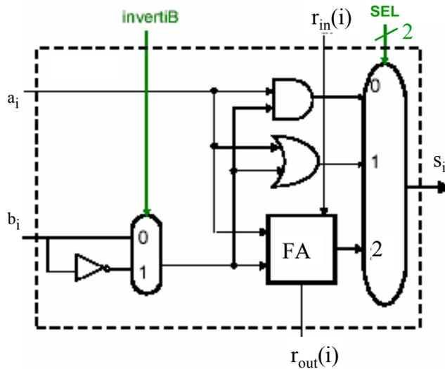
$r_{in}(i) = r_{out}(i-1)$   $i = 1, 2, 3, \dots, 31$   $i \neq 0$
