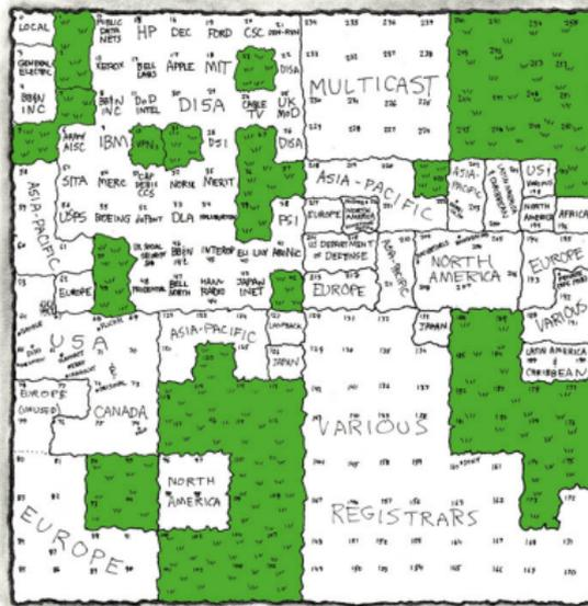
THIS CHART SHOWS THE IPv4 ADDRESS SPACE ON A PLANE USING A FRACTAL MAPPING WHICH PRESERVES GROUPING-- ANY CONSECUTIVE STRING OF IPv4s WILL TRANSLATE TO A SINGLE COMPACT, CONTIGUOUS REGION ON THE MAP. EACH OF THE 256 NUMBERED BLOCKS REPRESENTS ONE /8 SUBNET (CONTAINING ALL IPv4s THAT START WITH THAT NUMBER). THE UPPER LEFT SECTION SHOWS THE BLOCKS SOLD DIRECTLY TO CORPORATIONS AND GOVERNMENTS IN THE 1990s BEFORE THE RIRs TOOK OVER ALLOCATION.
