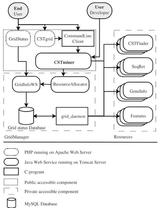
Fig. 1. The CSTgrid distributed software architecture.
