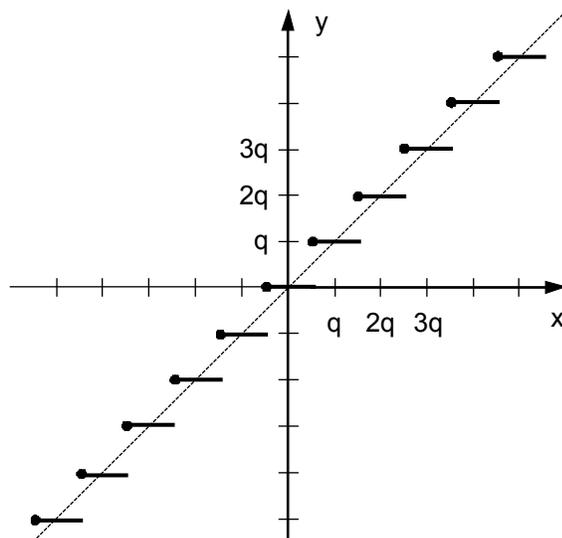
In Figure 10, the symbol “q” refers to the quantization step, i.e., the resolution of the data type.
