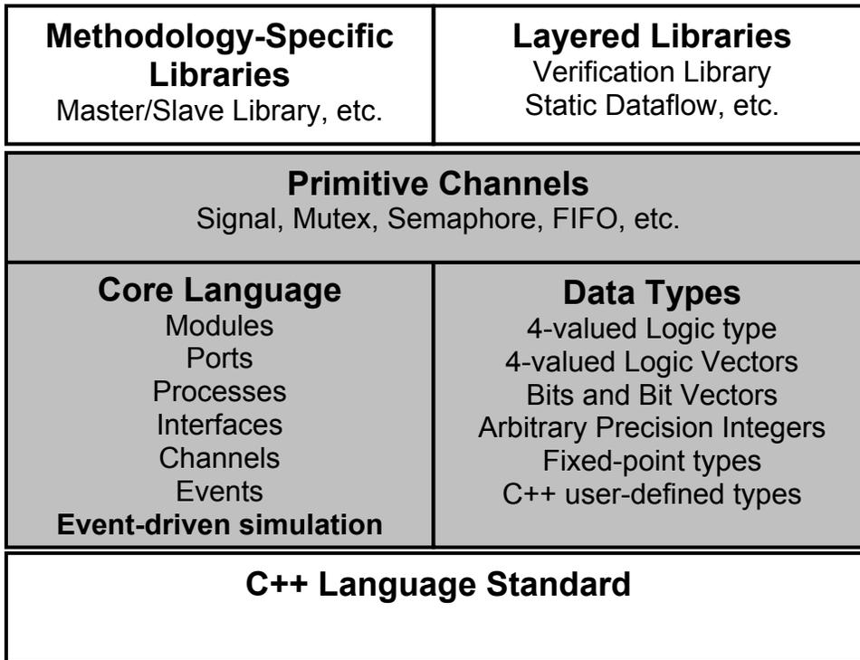
Figure 1 shows the SystemC language architecture. The blocks shaded with gray are part of the SystemC core language standard. SystemC is built on standard C++. The layers above or on top of the SystemC standard consist of design libraries and standards considered to be separate from the SystemC core language. The user may choose to use them or not. Over time other standard or methodology specific libraries may be added and conceivably be incorporated into the core language.
