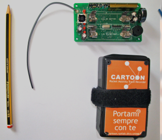
Circuitry and package of a PMTR. In the packed version, the antenna is fixed all around the box, to avoid accidental disconnections
