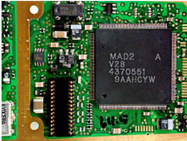
The microprocessor on the circuit board in the cell phone. http://electronics.howstuffworks.com/cell-phone6.htm
