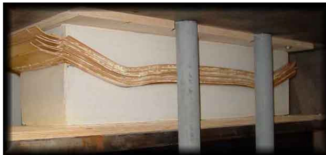
Figure 2.2.2: Maple veneers in a hydraulic press
