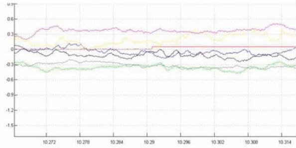
Fig 8. Typical graph of the signals before and during a LED pulse. Red channel: LED; gray and lilac channels: optically/electrically shielded neural basin; yellow and green channels: non-shielded neural basin; other channels: non-shielded control basin.
