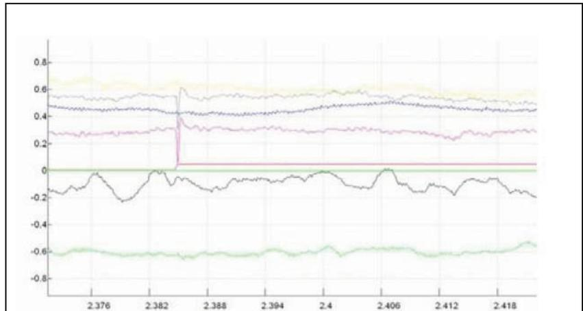
*Fig. 5. Phase b) graph of the signals before and during a laser pulse. The laser source is covered with a double aluminium foil. Red channel: laser; gray and lilac channels: neural basin, shielded by brass Faraday cage, plastic/aluminium cap, cardboard box; other channels: control basins, put inside the brass Faraday cage, one free and the other inside a cardboard box.*
