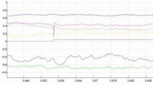
*Fig. 6. Phase c): graph of the signals before and during a laser pulse. The laser is more than 1 meter apart and directed to an opposite direction. Red channel: laser; gray and lilac channels: neural basin, shielded by brass Faraday cage, plastic/aluminium cap, cardboard box; other channels: control basins, put inside the brass Faraday cage, one free and the other inside a cardboard box.*
