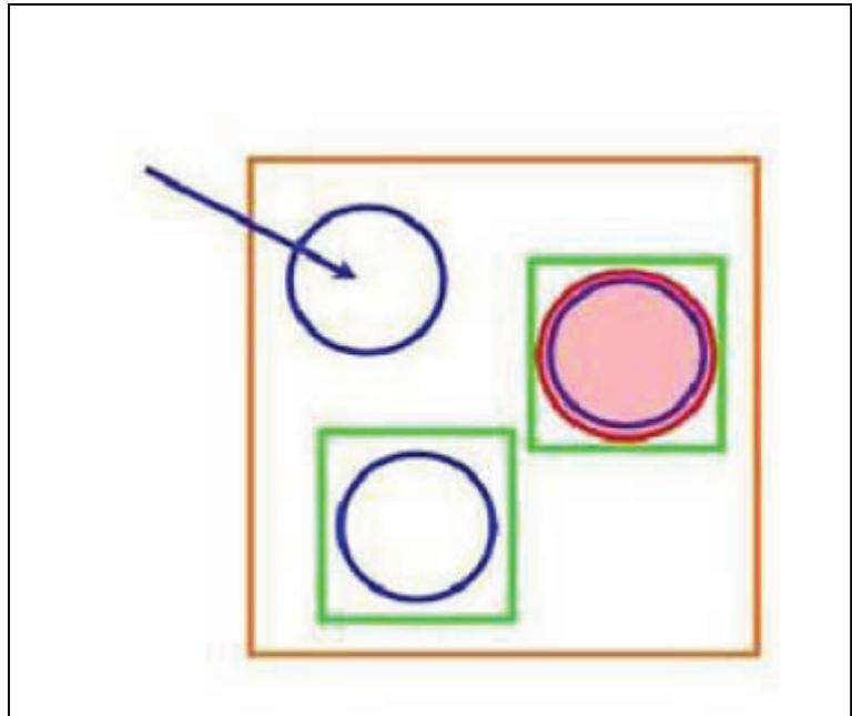
*Fig. 2. Schema of the experiment . The three basins are closed into a brass Faraday cage (yellow square). One basin is hit by the laser (blue arrow), one is inserted in a cardboard box (green square), the third one is covered by a thick plastic cap (red circle) wrapped with a double aluminium foil and inserted in a cardboard box.*
