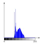
▶ The histogram components are localized in a narrow region of the intensity values.
