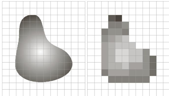
The image observed by the acquisition device is projected onto the sensor array (a) where it is sampled and quantized (b).
