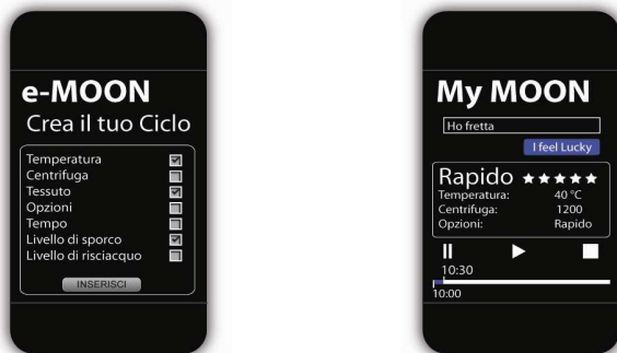
Figure 3 e-Moon and My Moon user interfaces. In the figure on the right the MP3-like stop and delay function is visible
