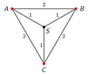
The minimum tree spanning the special vertices is not necessarily optimal (and it might not even exist)
