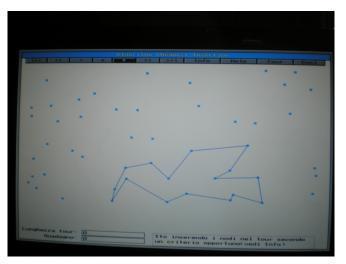
Add at each step the node that minimally increases the circuit cost
