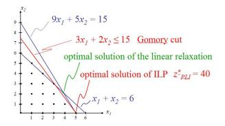
In this case, reoptimization leads to an integer solution (5,0), which is optimal for the original *ILP* problem, with  $f^* = 40$
