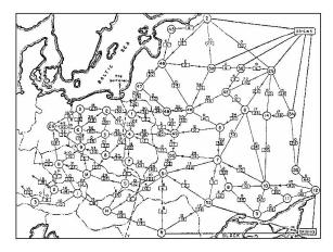
Find the bottleneck: links to destroy in order to reduce the flow Conversely, select the links to improve in order to increase the flow
