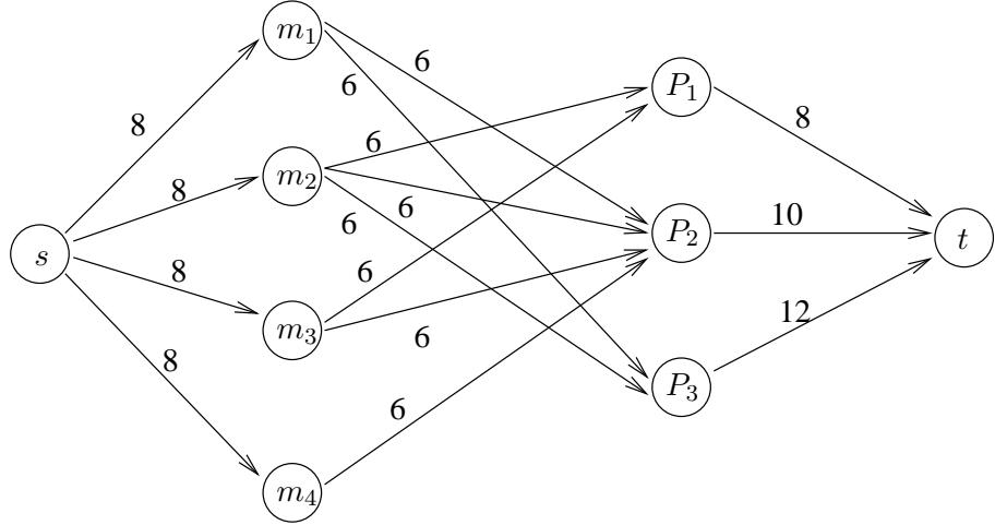
All arcs outgoing from  $s$  have capacity 8, equivalent to the number of available engineers per month. All arcs connecting month-nodes to project-nodes have capacity 6, as no more than 6 engineers can work on the same project in the same month. All arcs incident in  $t$  have capacity equivalent to the number of man-months needed to complete the project.
