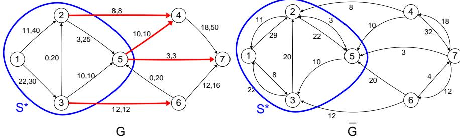
No more augmenting paths can be found. The minimum cut is highlighted in red, induced by  $S^* = \{1, 2, 3, 5\}$ . It has total capacity  $k(S^*) = \varphi = 33$ .
