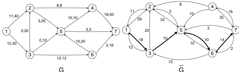
Observe that all augmenting paths for this network use the backward arc  $(5, 6)$ . From the flow point of view, this amounts to unload arc  $(6, 5)$ , decreasing the amount of product flowing through it.
