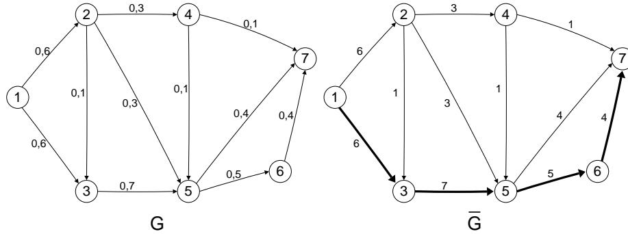
We sent  $\delta = 4$  units on path 1-3-5-6-7.  $\delta$  is given by arc  $(6, 7)$ , which has the smallest capacity  $k_{ij}$  of the path.
