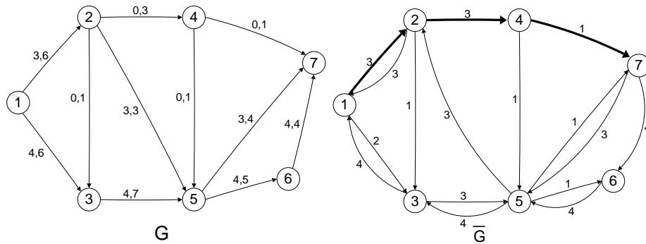
We sent  $\delta = 1$  units on path 1-2-4-7.  $\delta$  is given by arc (4, 7). We obtain a flow of value  $\varphi = 8$ .
