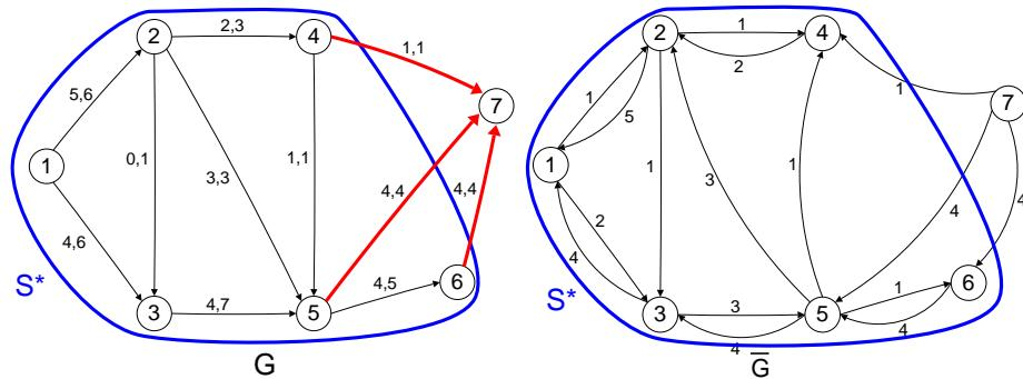
No augmenting paths can be found in  $\bar{G}$  and the algorithm halts. The set  $S^* = \{1, 2, 3, 4, 5, 6\}$ , highlighted in blue, indicates the nodes that can be reached from the source 1 in  $\bar{G}$ .  $S^*$  induces the minimum cut corresponding to the flow  $\underline{x}$ , which is highlighted in red. Correctness can be checked by observing whether the value of the flow equals the total capacity of the cut. At any optimal solution, the two values must be equivalent.
