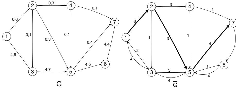
We sent  $\delta = 3$  units on path 1-2-5-7.  $\delta$  is given by arc  $(2, 5)$ , which has the smallest residual capacity  $\bar{k}_{ij}$  of the path. We obtain a flow of value  $\varphi = 7$ .
