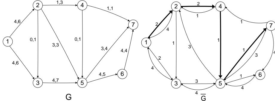
Se send  $\delta = 1$  units on path 1-2-4-5-7.  $\delta$  is given by arc (4, 5) (or (5, 7)). We obtain a flow of value  $\varphi = 9$ .
