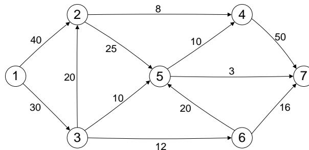
find a maximum flow from node 1 to 7, starting from a feasible flow of value 10, obtained by sending 10 units on the path 1-3-6-5-4-7. Show the corresponding minimum cut.
