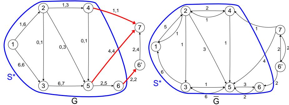
No more augmenting paths can be found. The minimum cut is highlighted in red, induced by  $S^* = \{1, 2, 3, 4, 5, 6\}$ . It has total capacity  $k(S^*) = \varphi = 7$ .
