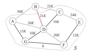
**Termination** Now, the subgraph is spanning (S = V), so that the algorithm terminates. The following figure reports he result, whose total cost is  $c_X = \sum_{ij} c_{ij} x_{ij} = 6\,800\,000$  euros.
