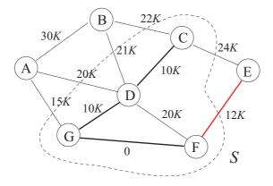
**Iteration 5** The cut induced by S contains edges (A, G) (with  $c_{AG} = 15K$ ), (D, G) (with  $c_{DG} = 10K$ ), (D, F) (with  $c_{DF} = 20K$ ) and (E, F) (with  $c_{EF} = 12K$ ). The cheapest one is (D, G), so that  $X := \{(F, G), (D, G)\}$  e  $S := \{D, F, G\}$ .
