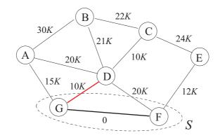
**Iteration 3** The cut induced by S contains edges (A, G) (with  $c_{AG} = 15K$ ), (D, G) (with  $c_{DG} = 10K$ ), (D, F) (with  $c_{DF} = 20K$ ) and (E, F) (with  $c_{EF} = 12K$ ). the cheapest one is (D, G), so that  $X := \{(F, G), (D, G)\} \in S := \{D, F, G\}$ .
