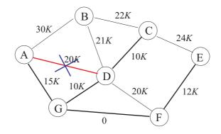
**Iteration 7** The seventh edge is (D, F), with cost  $c_{DF} = 20K$ . It induces cycle (D, F, G), so that it is discarded. In fact, vertices D and F both refer to representative C.
