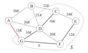
**Iteration 6** The cut induced by S contains edges (A, G) (with  $c_{AG} = 15K$ ), (D, G) (with  $c_{DG} = 10K$ ), (D, F) (with  $c_{DF} = 20K$ ) and (E, F) (with  $c_{EF} = 12K$ ). The cheapest one is (D, G), so that  $X := \{(F, G), (D, G)\}$  e  $S := \{D, F, G\}$ .
