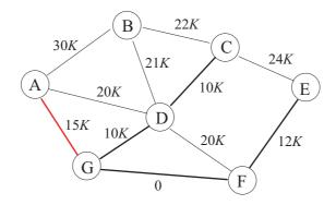
The auxiliary vector is updated appending component  $\{A\}$  to component  $\{C, D, E, F, G\}$ , since the former is smaller (one vertex versus five). We write C in position A and the (negative) sum of the two cardinalities -5 - 1 = -6 in position C.
