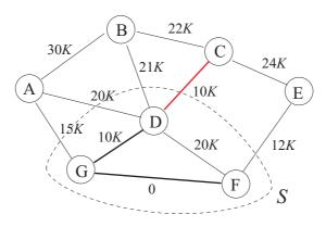
**Iteration 4** The cut induced by S contains edges (A, G) (with  $c_{AG} = 15K$ ), (D, G) (with  $c_{DG} = 10K$ ), (D, F) (with  $c_{DF} = 20K$ ) and (E, F) (with  $c_{EF} =$
