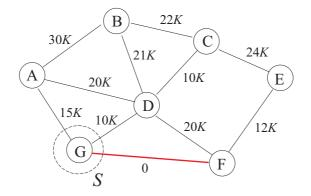
**Iteration 2** The cut induced by S contains edges (A, G) (with  $c_{AG} = 15K$ ), (D, G) (with  $c_{DG} = 10K$ ), (D, F) (with  $c_{DF} = 20K$ ) and (E, F) (with  $c_{EF} = 12K$ ). The cheapest one is (D, G), so that  $X := \{(F, G), (D, G)\}$  e  $S := \{D, F, G\}$ .
