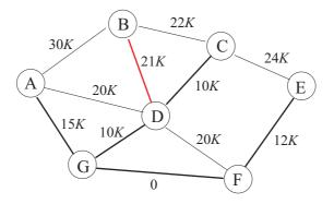
The auxiliary vector is updated appending component  $\{B\}$  to component  $\{A, C, D, E, F, G\}$ , since it is smaller (one vertex versus six). We write C in position B and the (negative) sum of the two cardinalities -6 - 1 = -7 in position C.
