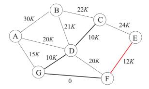
The auxiliary vector is updated appending component  $\{E\}$  to component  $\{C, D, F, G\}$ , since the former has smaller cardinality (one vertex versus four). We write C in position E and the (negative) sum of the two cardinalities -4-1 = -5 in position C.
