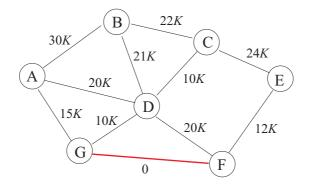
After adding the new edge, the auxiliary vector is updated appending component  $\{G\}$  to component  $\{F\}$ . The two components have the same cardinality, so that the choice is arbitrary. In order to perform the append, one writes F in position G and writes the (negative) sum of the two cardinalities -1 - 1 = -2in position F:
