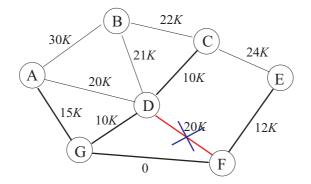
**Iteration 8** The eighth edge is (B, D), with cost  $c_{BD} = 21K$ . It does not induce any cycle, so that it is added to the solution. In fact, vertex B is isolated, whereas vertex D refers to vertex C, which is a representative.
