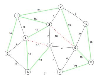
2.3 **Optimality proofs**. It suffices to verify that there exists a diminishing edge. By inspection, we observe that, by adding edge (1,5) to the tree, the cycle (1,5,4,3,2,1) is introduced. In such cycle, edge (4,3) has a strictly larger cost than (1,5).
