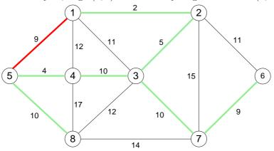
Therefore, by removing edge (4, 3) and adding edge (1, 5), a spanning tree of strictly smaller total cost is obtained. It is shown in the following figure.
