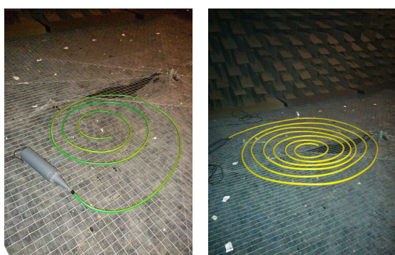
(c) Short narrow tube (length 8.8 m, inner diameter 1.2 cm). (d) Long medium-sized tube (25 m, 1.9 cm).
