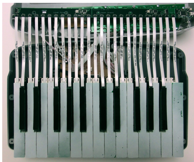
Figure 2. Two octaves of keys with controller board (top), mounted on a MIDI keyboard.
