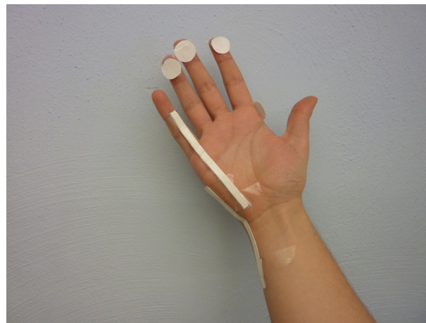
Figure 4. Paper replicas of sensors used in a workshop. The positions of the replicas were found through experimentation, unhindered by risk of damage to the actual sensors.
