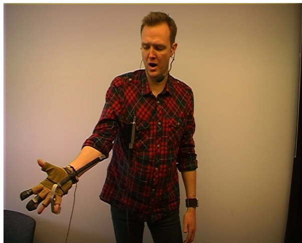
Figure 5. A singer performing an aria using gesturally controlled signal processing in the final test in the prototyping process of designing the Throat V3.
