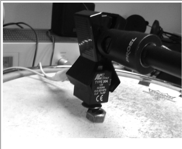
Figure 10. Testing a solenoid on a snare drum.
