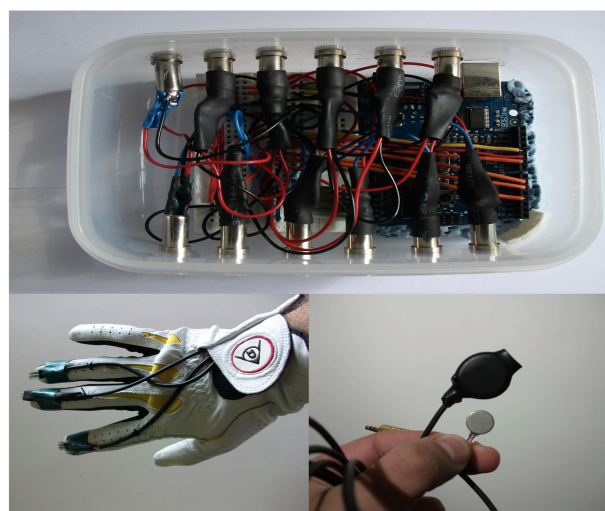
Figure 2. (Top) Inputs and outputs of the Arduino prototype box, (bottom left) glove with pressure sensors attached and (bottom right) vibrating motors with and without rubber shield.
