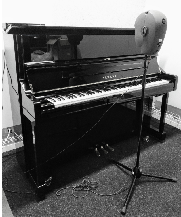
Figure 1: The binaural recording setup used in Zurich. The piano lid is in ‘semi-open’ position
