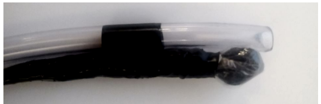
Figure 3: Resin's mouthpiece, consisting of the sound tube and the Lavalier microphone
