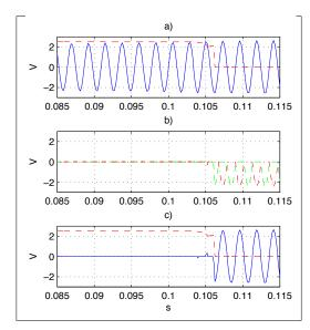
**Figure 5.** Spice simulation of the circuit excited with a sinusoidal signal with slowly increasing amplitude. a) input signal (blue solid line) and the voltage  $V_p$  (red dotted line); b) voltages at the two anodes of the twin diode 6H6; c) output signal (blue solid line) and the voltage  $V_p$  (red dotted line). The selector is turned on  $C_2 = 0.1 \mu F$ .
