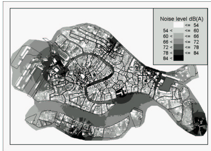
Fig. 2. The Existing Siren Allocation in Venice and a SoundPLAN simulation of the generated sound pressure.
