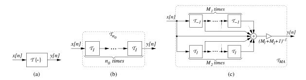
**Figure 1.2:** Block schemes of discrete-time systems; (a) a generic system  $\mathcal{T}\{\cdot\}$ ; (b) ideal delay system  $\mathcal{T}_{n_0}$ ; (c) moving average system  $\mathcal{T}_{MA}$ . Note the symbols used to represent sums of signals and multiplication by a constant (these symbols will be formally introduced in Sec. 1.6.3).
