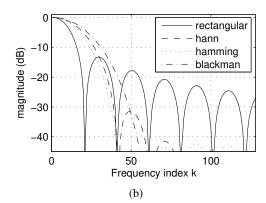
**Figure 1.13:** Comparison of different windows; (a) time-domain window sequences, symmetrical with respect to n = 0; (b) window spectra in the vicinity of k = 0. Differences in terms of main lobe width and relative side lobe level can be appreciated.
