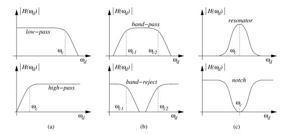
**Figure 1.17:** Classification of filters into basic categories, depending on their magnitude response  $|H(\omega_d)|$ : (a) low-pass and high-pass filter; (b) band-pass and band-reject filter; (c) resonator and notch filter.
