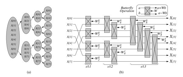
**Figure 1.11:** (a) Tree of calls in an invocation of RECURSIVE-FFT: the leaves contain a bit-reversal permutation of x[n]; (b) parallel realization of ITERATIVE-FFT, where butterfly operations involve bit-reversed elements of x[n].
