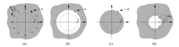
**Figure 1.14:** Pole-zero plots and ROCs of some simple transforms: (a) finite-length exponential sequence; (b) right-sided exponential sequence with |a| > 1; (c) left-sided exponential sequence with |a| > 1; (d) exponentially damped, right-sided sinusoidal sequence. In all plots the dotted circle is the unit circle and the gray-shaded region is the ROC of the corresponding transform.
