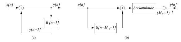
**Figure 1.4:** Block schemes for constant-coefficient difference equations representing (a) the accumulator system, and (b) the moving average system.
