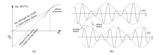
**Figure 1.15:** Comparing phase delay and group delay: (a) evaluation of phase delay and group delay for a generic non-linear phase response; (b) illustration of phase delay and group delay for a narrowband signal.
