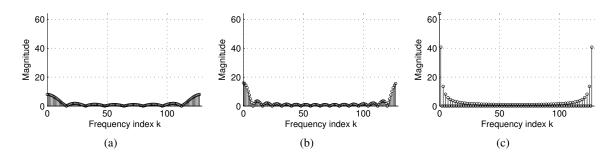
**Figure 1.10:** Examples of DFT (N = 128) applied to a rectangular window: (a) M = N/16, (b) M = N/8, (a) M = N/2.
