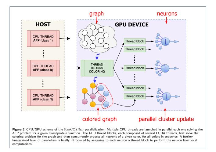
stream, where a CUDA stream is a queue of commands or operations that are executed in a specific order; while operations on a stream are executed sequentially, operations in different streams may be executed concurrently or out of order with respect to one another. In the specific case of PARCOSNET, kernel executions belonging to different AFP problems are interleaved and executed concurrently.
